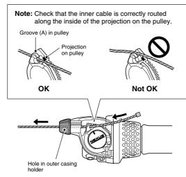
2) Hook the inner cable into groove (B) in the pulley, and pull the inner cable so that the inner cable drum fits into the hole (B) in the pulley. After this, insert the outer casing into the outer
